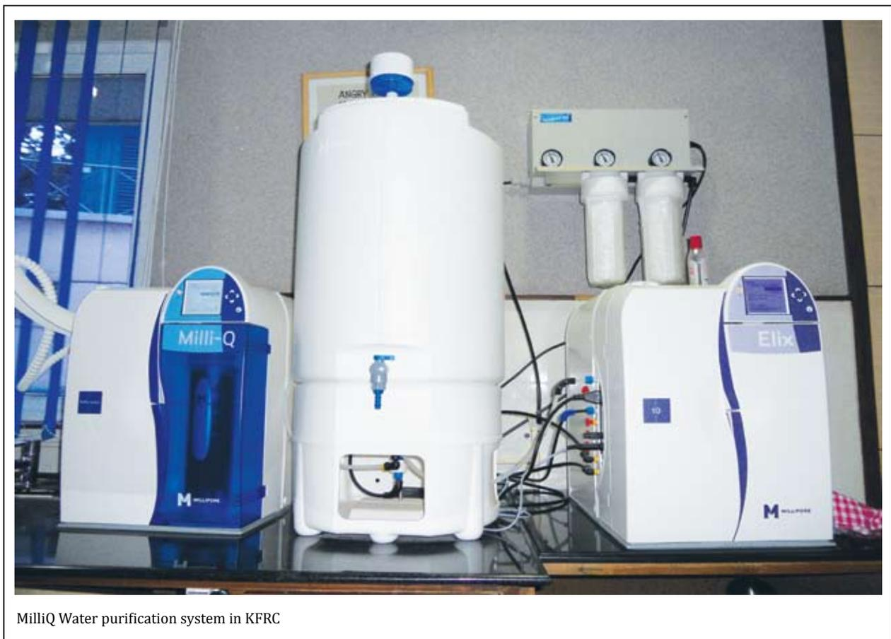
MilliQ Water purification system in KFRC
